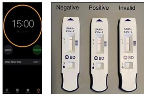
Read results after 15 minutes. One red line (C) - indicates a negative result. Two red lines (C and T) - indicates a positive result. One line (T) - is an invalid test (the test will need to be re-done).
